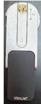
Vitrojet grid cassette. Grids are placed so that the foil is facing to the right
