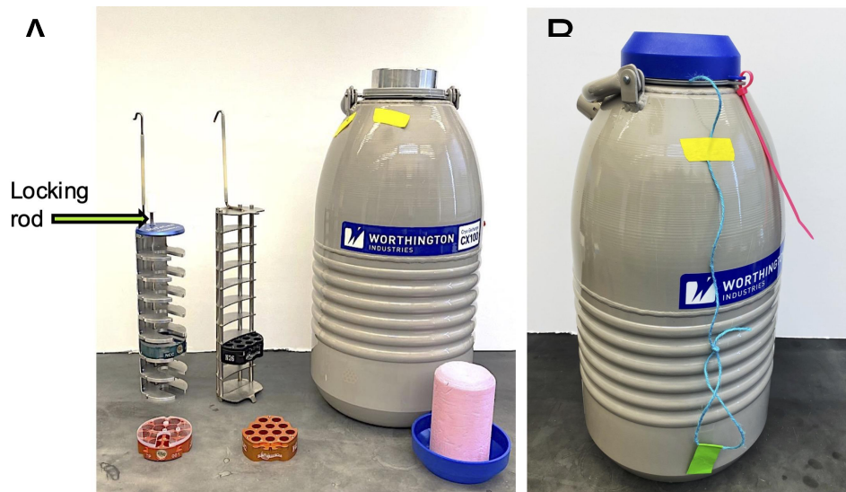
Figure 4. A) Puck canes hold pucks. MiTeGen cane (left) requires use of a locking rod to secure pucks. SubAngstrom pucks (middle) have magnets to secure them in the cane and do not require a locking rod. B) Dry shipper holding a conical tube secondary container. The string
