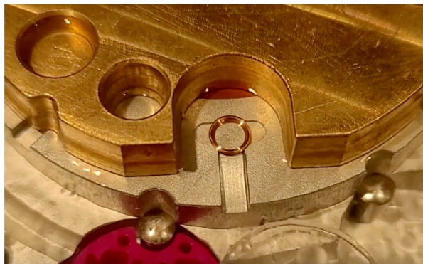
Figure 4. Clip ring sitting on the pedestal with the lip facing up, and brass plate open to the pedestal. This is ready for placement of a grid onto the clip ring.
