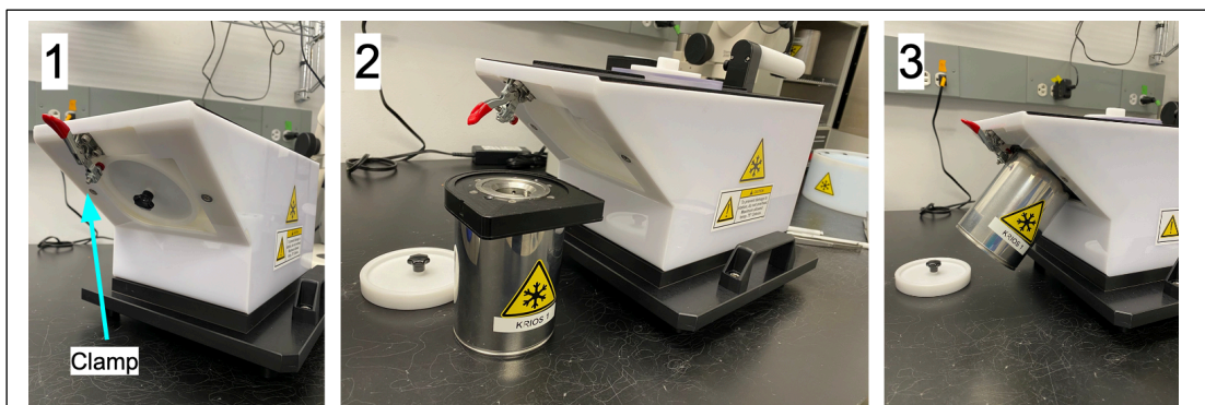
Figure 9. Proper procedure to attach NanoCab to transfer station. Use the clamp to secure the window cover when NanoCab is unattached.
