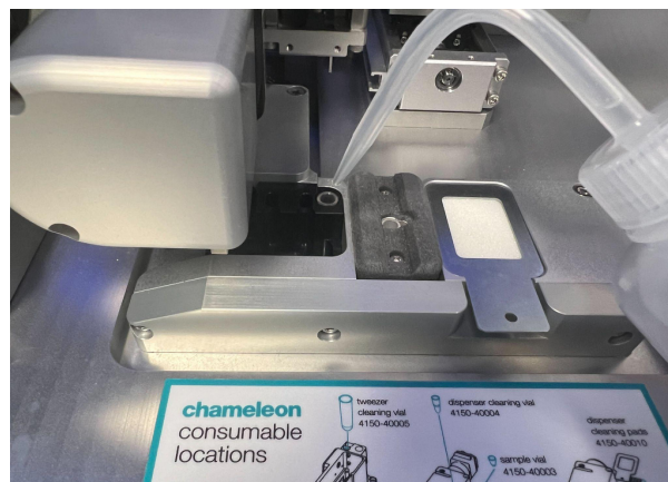
Figure 9. Use the squirt bottle to fill the dispenser cleaning vial with methanol.
