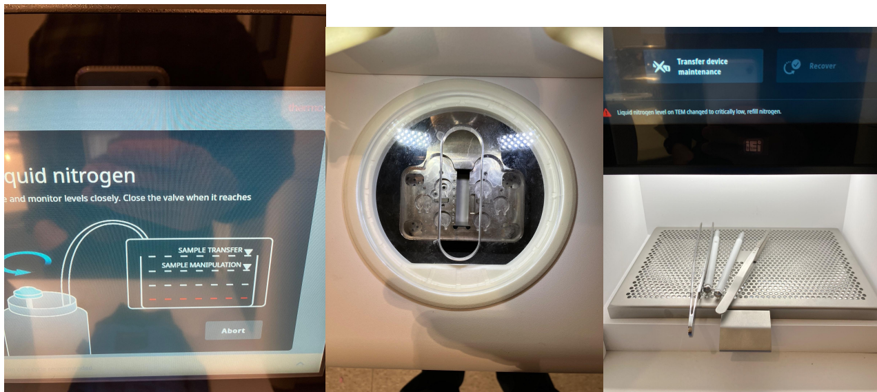
Figure 2: The cryo loading station. A) Screen during initial filling with liquid nitrogen. B) The window to the grid loading area.. C) The tool storage area.
