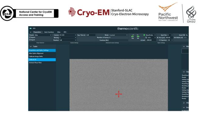
4.5.3.1 <u>IF</u> there is a beam shift, insert FluScreen. In **TEMUI Tune** tab, go to subsection **Direct** Alignments then select **Beam shift**. **DO NOT TOUCH GUN TILT AND GUN SHIFT**. <u>Proceed to 4.2.4 if no beam shift adjustment is needed</u>
