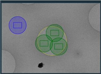
4.10.16 In the Autofocus Area Settings, set Recurrence to After Distance and input 8 μm. 4.10.17 Optional: Add Add Drift Measurement Area in the image display and specify Recurrence as Always
