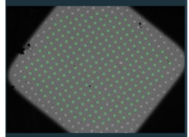
4.10.8 To remove multiple foil holes, select **Selection Brush**. Remove holes with contaminations or cracks. To add holes, hold "CTL" and click on the hole while **Selection Brush** is highlighted.
