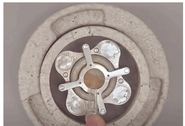
Figure 3. Ethane Holder Assembled. Proper ethane tip placement shown.
