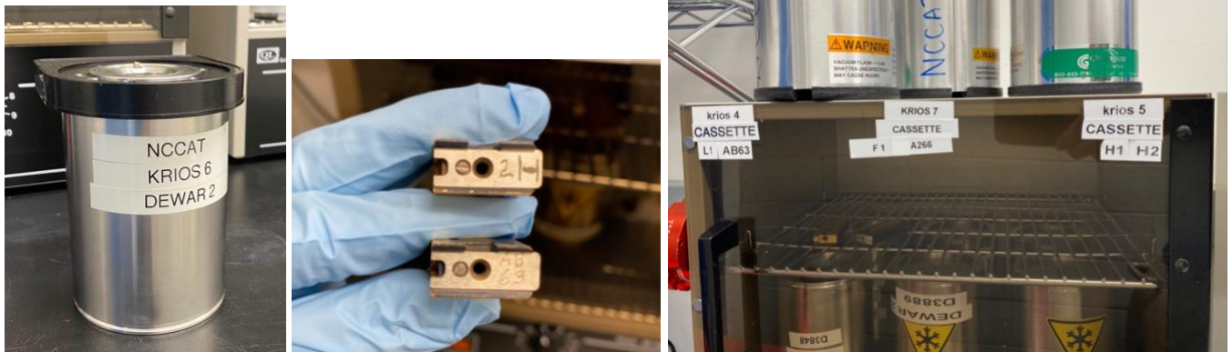
Figure 2. Labels clearly indicate which NanoCab and cassette are to be used for each microscope. A) Each NanoCab is labeled (here the NanoCab for Krios6 is shown). B) The silver end of the cassette has an etched label (here labels "H2:" and "AB63" are shown). C) Each oven is labeled with which NanoCabs and cassettes should be placed inside.
